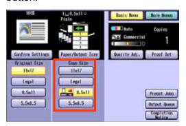
For the following procedure, refer to steps 5 to 6 of Basic Operation for the 2-Sided Copy Mode (see page 40). Ex: Combination of Letter (Portrait layout) and Ledger (Landscape layout) original Copy Images (1 -> 2 copy mode) Bind Position is SHORT EDGE
